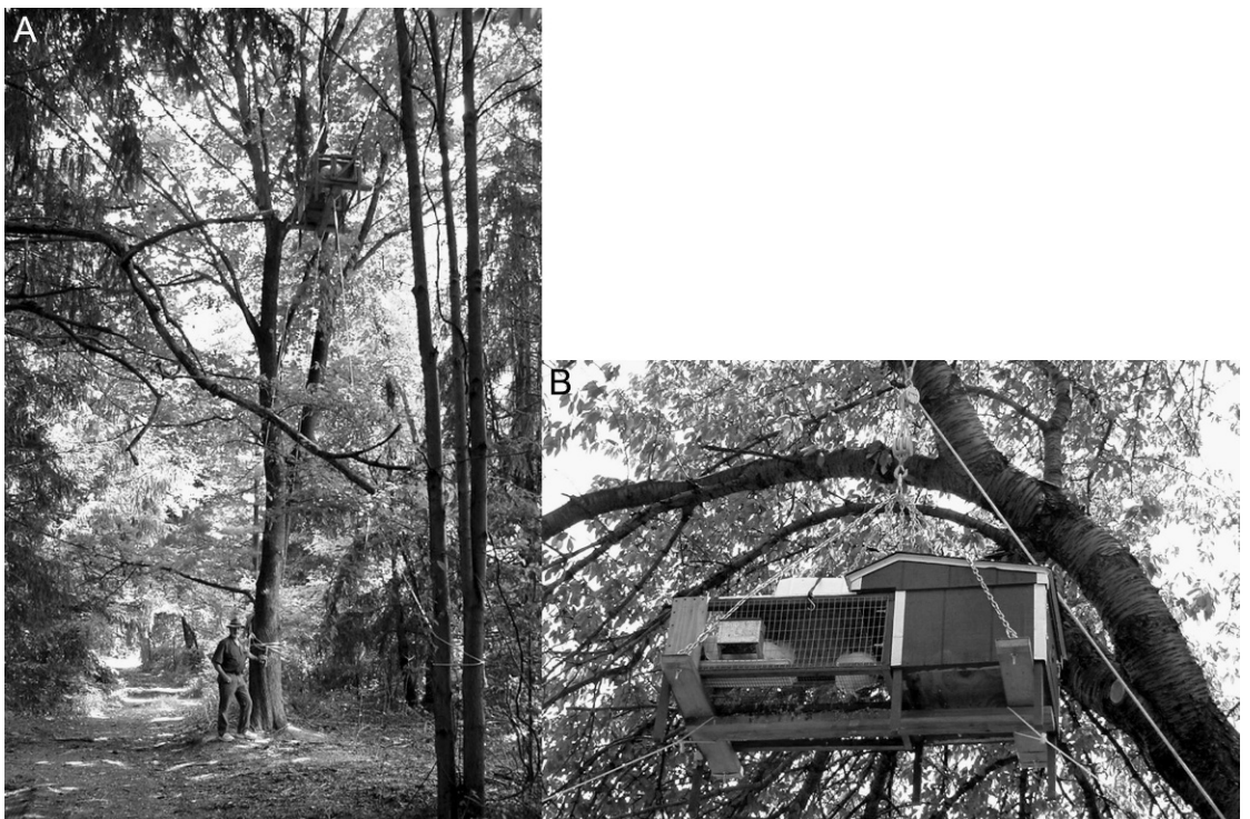
Fig. 2. (A) Elevating system for sentinel chicken surveillance in the canopy. (B) Enlarged view in canopy.
