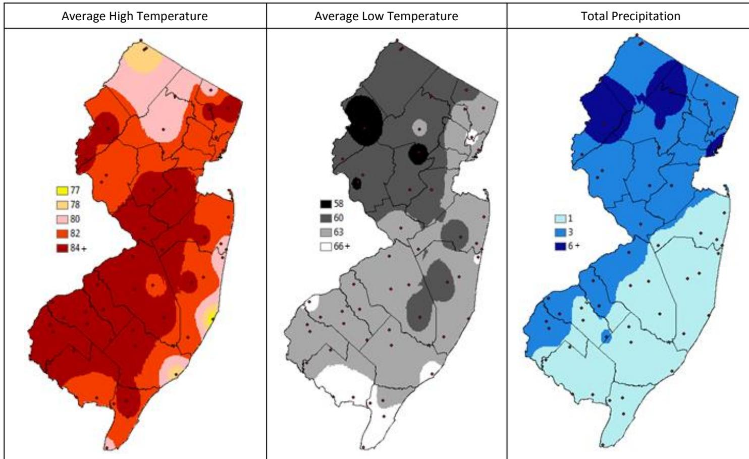
The three figures show the interpolation of average maximum (°F) and minimum temperature (°F) and total precipitation (inches) for 30 days prior to 8 July 2017 in New Jersey. Data points are from about 56 weather stations maintained through the New Jersey Weather & Climate Network and the State Climatologist. Interpolation between points was performed using ArcMap 10.1.
