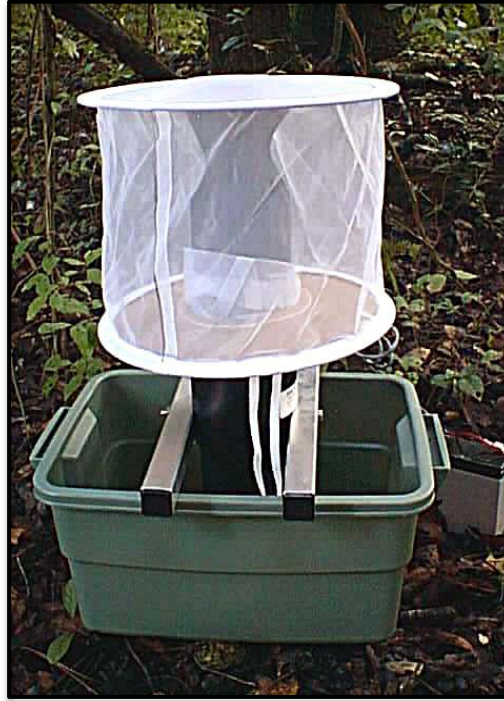
B. CDC Gravid traps baited with a hay infusion
